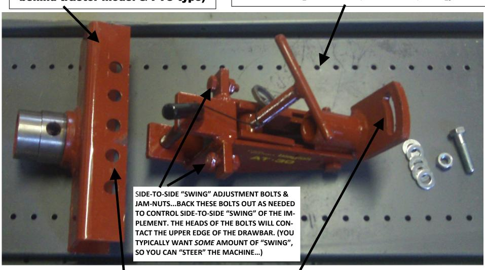
"OFFSET" HOLES in Drawbar, to allow slightly off-center use of Implement (Rarely utilized...most of time, the Tool Carrier is attached to the "center" hole) SLOTTED HÓLE allows the operator to angle the implement on a slightly different plane than the tractor axle (for working hillsides, etc.)
