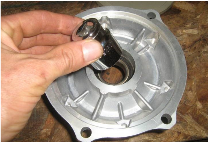
#9. SELECT PIECE OF PIPE, SOCKET, ETC. TO FIT IN BACK OF ENGINE MOUNTING FLANGE, UP AGAINST THRUST BEARING
