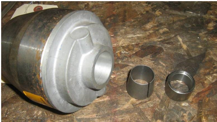
#13. NEW STYLE CLUTCH INCLUDES (FROM LEFT): CLUTCH, SPLIT TAPER-LOCK BUSHING, AND SPACER. MAY ALSO INCLUDE AN ALLEN WRENCH.
