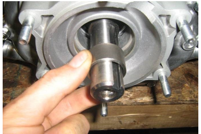
#14. SLIDE SPACER ONTO ENGINE CRANKSHAFT
