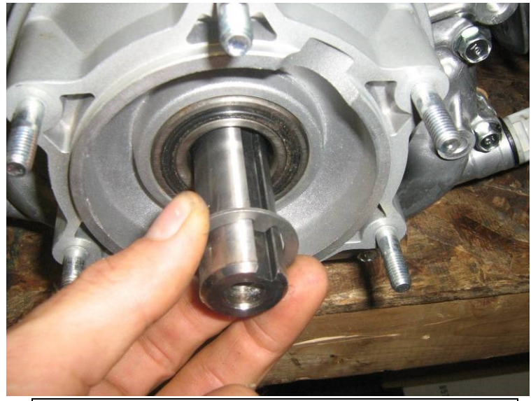
#6. REMOVE THRUST WASHER FROM CRANKSHAFT
