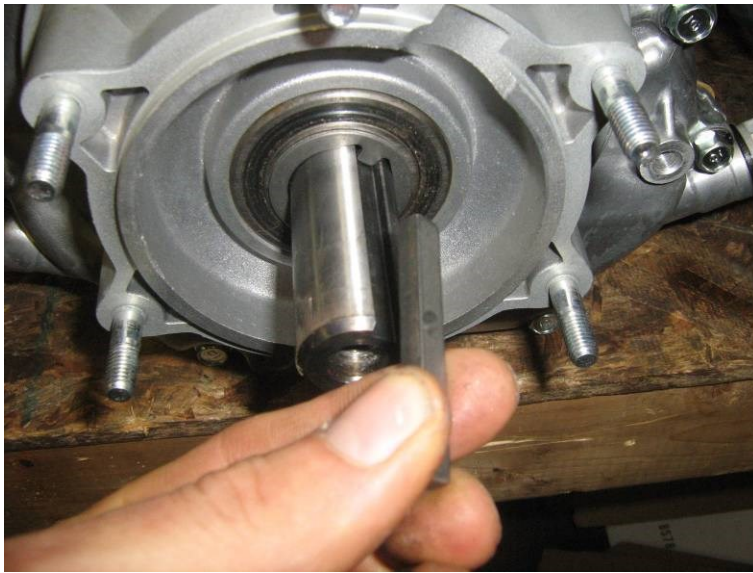
#5. REMOVE KEY FROM CRANKSHAFT
