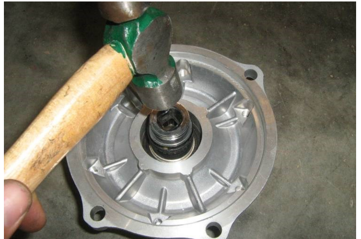
#10. DRIVE BEARING OUT OF ENGINE MOUNTING FLANGE
