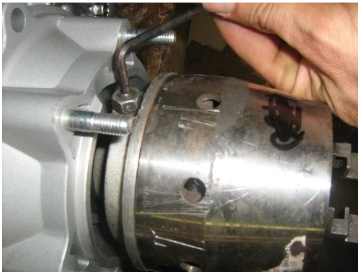
#3. LOOSEN ALLEN-HEAD SET SCREW WITH 4MM ALLEN WRENCH
