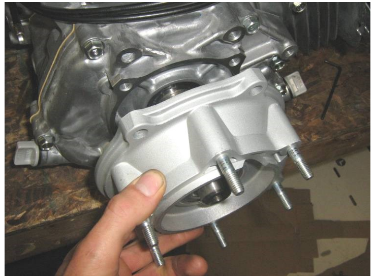
#8. REMOVE ENGINE MOUNTING FLANGE FROM ENGINE
