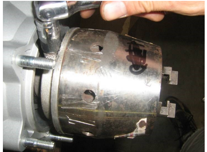
#2. LOOSEN JAM-NUT WITH 13MM SOCKET
