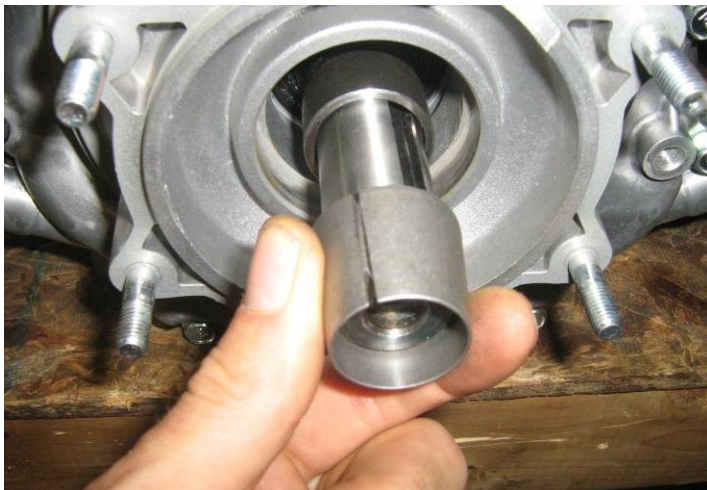
#15. SLIDE SPLIT TAPER-LOCK BUSHING ONTO CRANKSHAFT, BIG END FIRST
