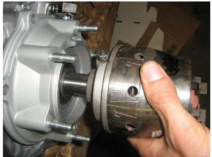
#4. REMOVE CLUTCH FROM ENGINE SHAFT
