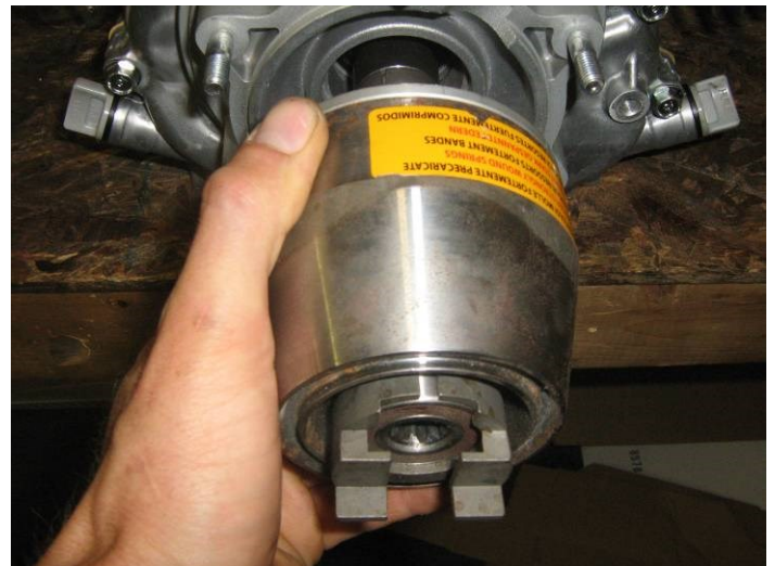
#16. SLIDE NEW CLUTCH ONTO ENGINE CRANKSHAFT
