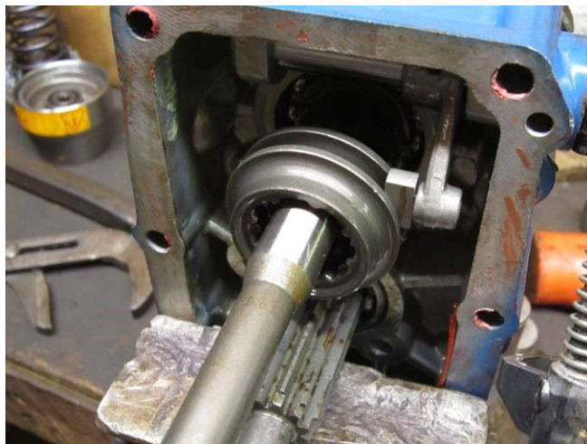
14. BY PUSHING THE PTO ENGAGEMENT LEVER, YOU CAN NOW "POP" THE PTO SLIDER GEAR OFF THE LOWER SHAFT. NOTE: IT'S BEST TO DRAPE A RAG OVER THE HOUSING BEFORE DOING THIS, BECAUSE THE 'DETENT BALLS' CAN GO FLYING WHEN THIS GEAR IS POPPED OFF...THE RAG KEEPS YOU FROM LOSING THEM!
