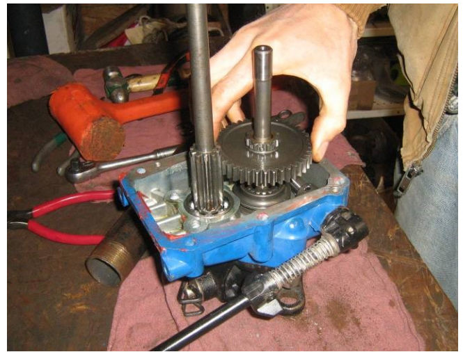
13. THE LARGE PTO DRIVE GEAR CAN THEN BE REMOVED. (NOTE HOW IT COMES OFF...YOU CAN PUT IT BACK ON UPSIDE-DOWN IF YOU'RE NOT PAYING ATTENTION!! WILL NOT WORK!! )
