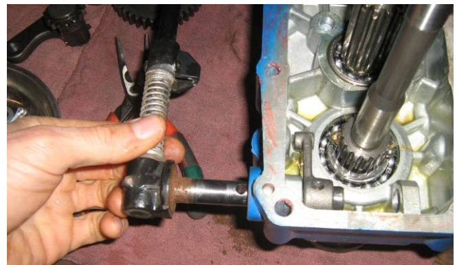
17. REMOVE THE EXTERNAL SHIFTER LEVER. YOU MAY HAVE TO ROTATE IT BACK AND FORTH TO SLIP IT OUT OF THE INTERNAL LEVER IF IT'S A TIGHT FIT.
