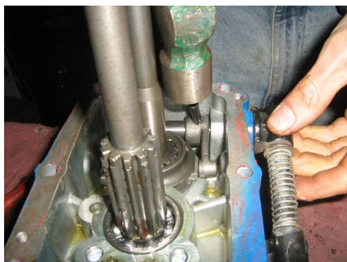
33. START ROLL PIN INTO HOLE...
