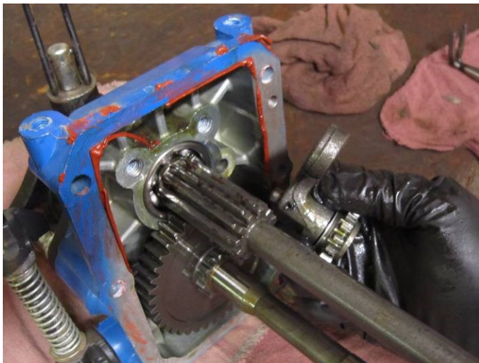
12. REMOVING REVERSER SPUR GEAR ASSEMBLY. NOTE THAT IT HAS A LOCATION PIN TO CENTER IT UP IN THE HOUSING, WHICH HAS TO BE PROPERLY FITTED INTO ITS HOLE UPON RE-ASSEMBLY.
