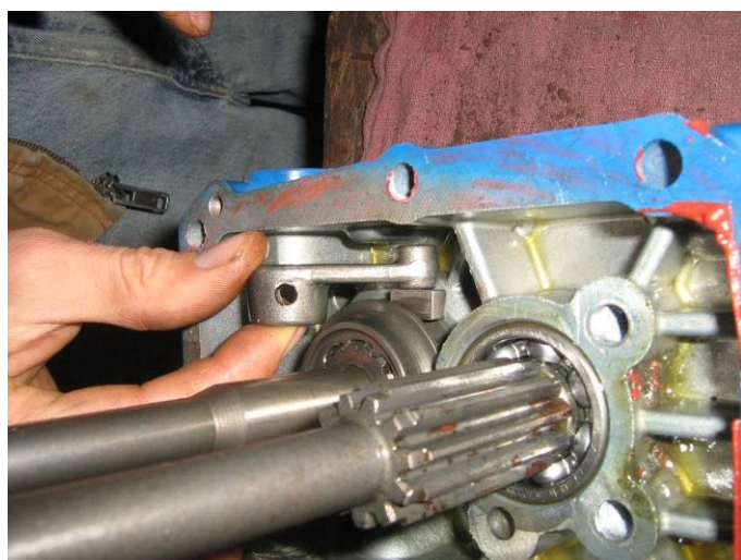
31. SET INTERNAL PTO LEVER DOWN INTO HOUSING, ENGAGING SHOE INTO GROOVE IN SLIDER
