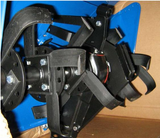
OVERLAPPING: Tines “stack” on top of each other, sharing common mounting bolts. 4 bolts per full set of 4 tines.
