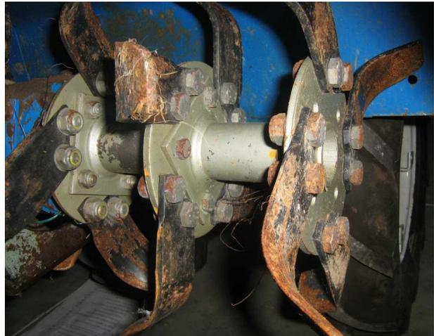
INDIVIDUAL: Tines bolt on individually, not sharing any mounting bolts. 8 bolts per full set of 4 tines.
