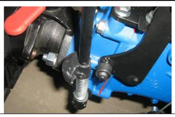
TRACTOR PTO LEVER STILL **NOT** FULLY ENGAGED...THIS IS ONLY THE "FIRST CLICK" IN IT'S POSSIBLE MOVEMENT. IN THIS POSITION, IT **WILL** POP OUT OF GEAR UNDER LOAD AND EVENTUALLY DAMAGE THE PTO ENGAGEMENT GEARS IN THE TRANSMISSION.
