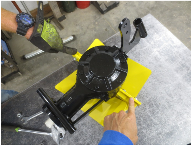
7. In this picture, we are pointing at the 2 “grass cutting blades” at the top of the plowshare/hub assembly (they are just squared-off steel blocks, they are not actually sharp)
