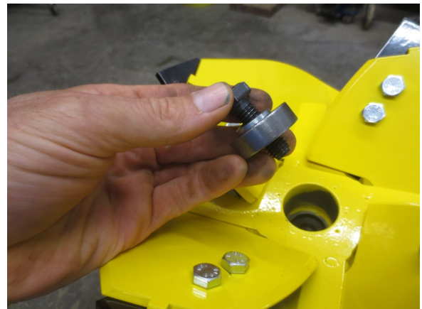
12. Remove the center bolt, lockwasher and thick washer
