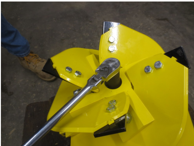
11. Using a 19mm or 3/4” socket, remove the center bolt (standard thread...lefty-loosey). If needed, block the hub with a piece of wood to keep it from turning
