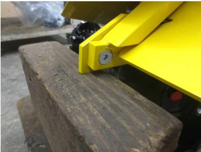
9. Detail showing “blade” supporting the plow (both sides should look like this) Make sure to have everything on a HARD surface...concrete is best.
