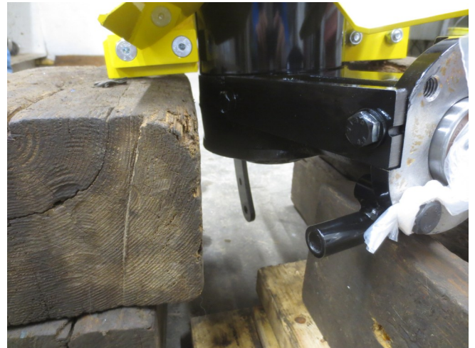
8. Flip the plow over, and, using some wood or steel blocks, support the weight of the plow by the two “grass cutting blades” shown in the previous picture
