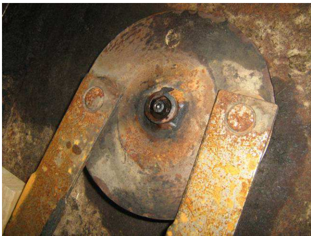
4A. If blade carrier is so tight on shaft that the above "pry-bar" method will not remove it, the following method will have to be used: After removing the original center bolt, replace it with a slightly LONGER bolt with an Allen (socket) head. DO NOT TIGHTEN!
