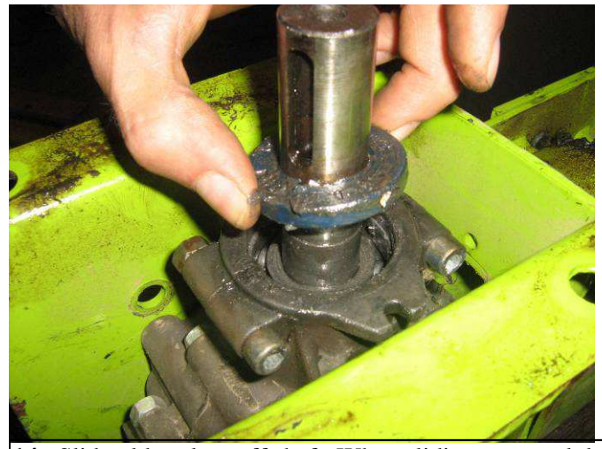
14. Slide old seal up off shaft. When sliding new seal down over shaft, MAKE SURE the inner lip of seal has been oiled , and take care not to cut the seal on the sharp edges of the key slot in the shaft. Tap new seal into place with a hammer, evenly on all sides, until flush with gearbox housing.
