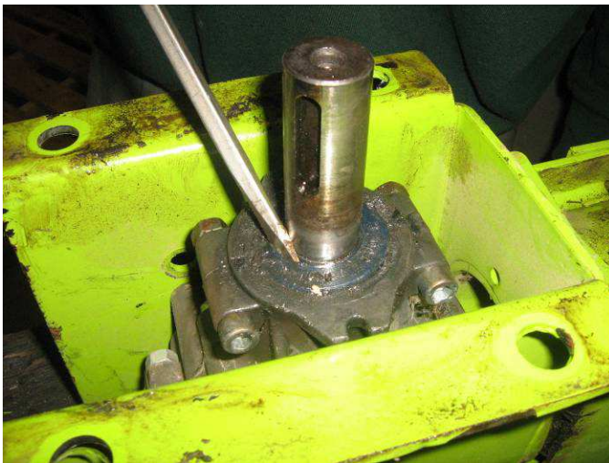
13. If either of the oil seals need to be replaced: Insert a flat-blade screwdriver slightly into the inner lip of the seal and pry it out of the gearbox. (this picture shows gearbox still in neck assy., and if replacing just the lower seal, this is fine. Obviously, replacement of the rear seal necessitates removal of the gearbox & U-joint.)
