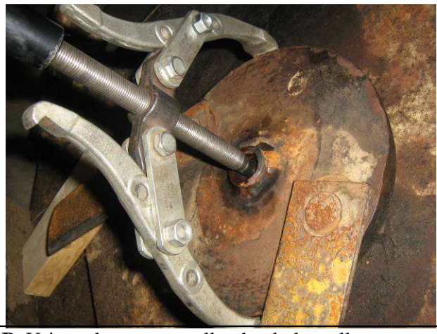
4B. Using a large gear-puller, hook the puller on outer edge of blade carrier and put center "pusher" bolt of gear puller in center of Allen-head bolt. This allows the puller to "push" against the shaft itself while pulling the blade. Make sure that if the blade carrier "bottoms out" against the Allen-bolt, you continue to back the bolt out or switch to a longer bolt if needed. You need to have AT LEAST 1/4" of threads screwed into the shaft to "push" against.
