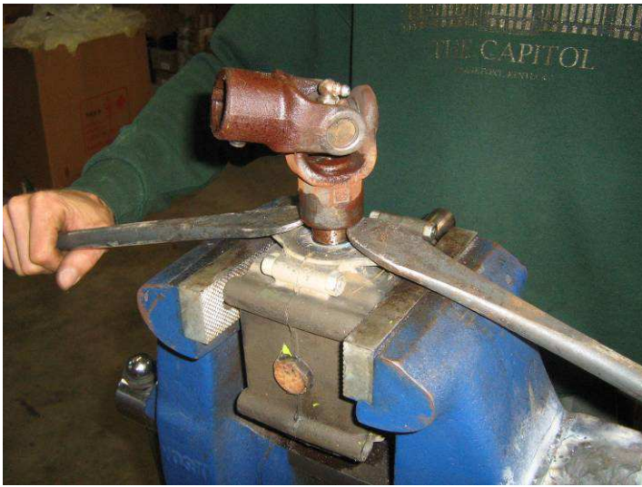
11. Using two pry-bars, pry U-joint up off of gearbox shaft (use even pressure on both sides).
