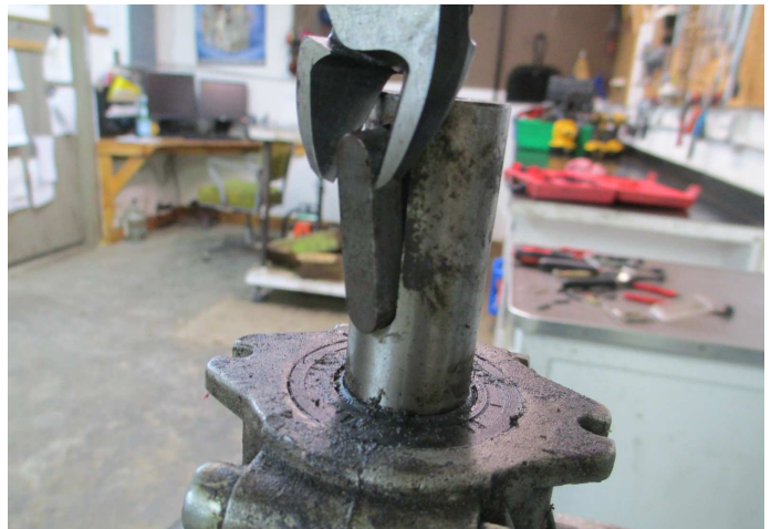
12. The easiest way to remove the keys from the shaft is to grip the edge of the key with a side-cuts (wire cutters) and leverage the cutters against the end of the shaft to pop the key out. If this makes a little burr on the key, you can file it off.
