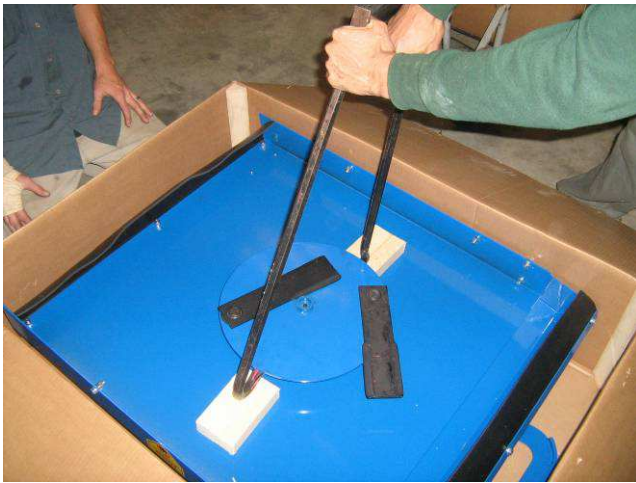
3. Using 2 pry-bars, pry up on blade carrier to get it off shaft. Apply EVEN pressure on both sides!
