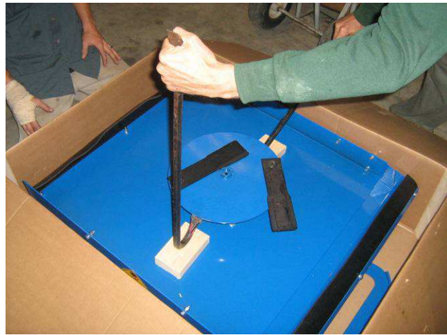
4. Blade carrier is coming up off shaft in picture. You may have to add additional wood pieces as it gets pried up, if it is "stiff" all the way off.
