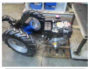
7. Engine & clutch removed from tractor. Note there are still a few wires hooked up. As long as you're careful, this works fine.
