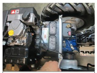
2. Remove battery retainer and cables with 10mm wrenches to remove battery from holding box. Remove negative cable FIRST!
