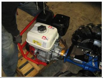
6B: If there is an implement on the tractor to "steady" the tractor, you can simply wiggle and slide the engine off the tractor, onto the support. (Gas engine pictured here...sorry, "stock" photo!
