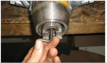
10. Now, even though the taper broke free, the clutch wiggles around, but it doesn't want to come off!! This is because there are still a few threads of the bolt holding. Put your Allen wrench back in the hole and unscrew the bolt.
