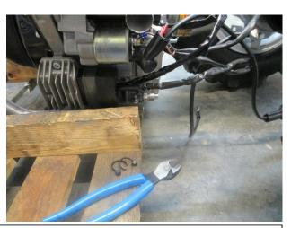
4. The voltage regulator can be unplugged to allow for more flexibility in removing the engine, OR the zip ties that bundle the wires together can be cut and then replaced later. This allows the engine to be "mostly free" of the tractor and give ample "slack" to maneuver the engine/tractor while removing the clutch. COMPLETE removal of the engine can be achieved by removing a few more wires, if you want. (if you do this, make sure you make notes on where they go!!
