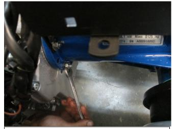
5. Proceed to remove the six nuts that hold the transmission flange to the engine's rear cover.
