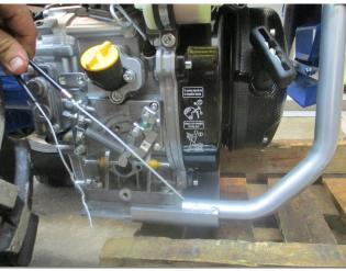
1. Remove throttle cable and operator presence control cable (OPC cable). Tag them, for proper re-assembly!! (NOTE the support under engine for ease of removal throughout process...a milk crate, cement block, or similar-sized object can be used)
