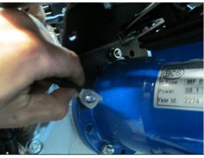
3. Negative side cable is fastened to an engine stud by a nut (13mm wrench) and requires removal (all these nuts have to come off anyway).
