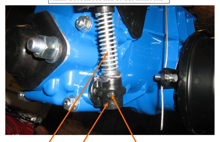
PTO Control Rod (has spring installed over it...some have this, some don't. The spring is actually useless, and can be discarded.
