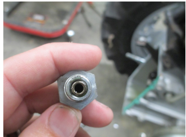
23a. This bolt is HOLLOW, and it houses a spring, which pushes on a detent ball...this is what "clicks" when you shift gears...
