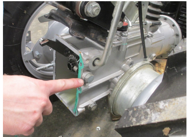
21. If you need to remove gears from the upper shaft (or the upper shaft itself), you'll first need to remove this bolt, which is the gearshift lever "detent" holder.
