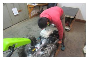
5) If you have help, one person can hold the engine in place while the other wiggles/pulls the tractor away from the engine. If you alone, just put the tractor in 1st or 2nd gear to keep it from rolling, and wiggle/pull the engine off.
