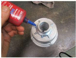
**10)** Reassembly is the reverse of removal. Make sure to apply a little bit of medium strength (blue) threadlocker to the (2) small set screws on the clutch before installation. Get the screws tight!! (If you are staring to worry that the Allen wrench will break, that's about tight enough!!)
