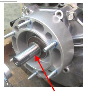
11) Make sure that the square "key" in the groove of the crankshaft is slid ALL THE WAY BACK as far as it will go toward the engine, as shown in this picture.
