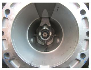
**12)** It is also good to apply a VERY SMALL AMOUNT of grease (multi-purpose) to the clutch fork pads that contact the throwout bearing plate on the clutch and also on the splined input shaft of the transmission. Then slide the engine & clutch back onto the tractor and tighten the 6 nuts.
