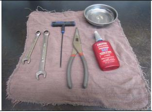
1) Typical tools needed: 10mm & 13mm wrenches, 2.5mm Allen wrench / key, needle nose pliers, medium strength (blue) threadlocker, magnetic tray
