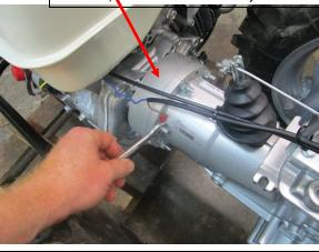
2) With the 13mm wrench, remove the (6) nuts and washers holding engine and adapter flange to transmission. If equipped with electric start engine, remove battery and battery cables. (REMOVE NEGATIVE CABLE FIRST!)
