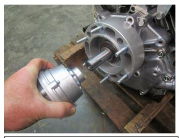
8) ... You are able to slide the clutch off of the engine's crankshaft. If the clutch has been in place a long time, there could be some corrosion preventing the clutch from sliding off easily; in this case, use a couple of prybars or large screwdrivers, and, placing one on each side (directly opposed to each other), pry the clutch off the engine.
