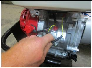
3) Pull the operator presence control (OPC)/kill switch wire bullet connectors apart where the single wire from the transmission goes into the engine's wiring harness.
