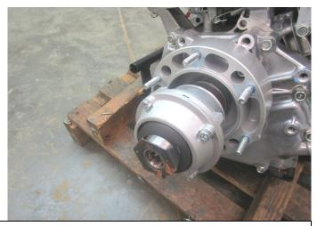
6) The clutch is affixed to the engine crankshaft. Pictured is the Grillo cone clutch for 1" keyed crankshaft engines (part number G 46875)...this fits Honda, Yamaha, Subaru, and other engines.
