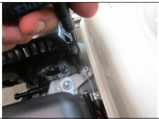
4) To detach the throttle cable form the engine, locate the end of the cable at the engine. On the Honda engines (pictured), it is next to the fuel tank/air filter, and the clamp is loosened using a 2.5mm Allen key. If equipped with a Subaru or Kohler engine, it may take a Philips head screwdriver. Also, if equipped with a Kohler or Yamaha engine, the throttle cable clamp is just underneath the front of the fuel tank.
