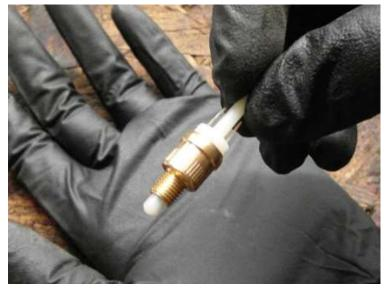
Switch. When they are BAD, the white plunger (shown on lower left side) typically sticks "in" periodically, which sticks it in the "off" position, and the engine will not run.
