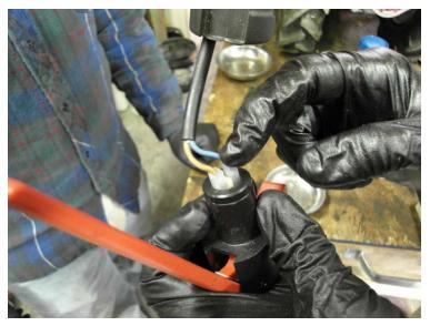
5) Install new switch, turning until tight, and reconnect wire terminals. It does not matter which wire goes on which connector of the switch.
