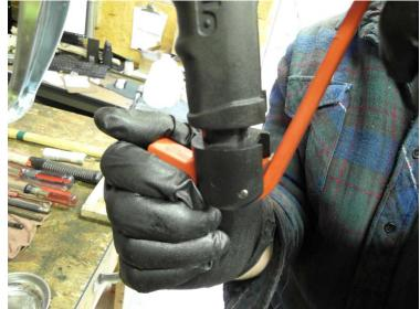
2) Twist back & forth a bit while pulling OPC lever assembly out of the end of the handlebar....it is tight!
