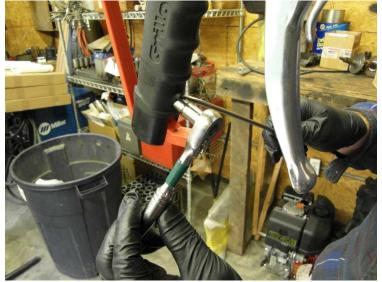
1) Remove screw holding OPC lever assembly onto the end of the handlebar with 7mm socket.
