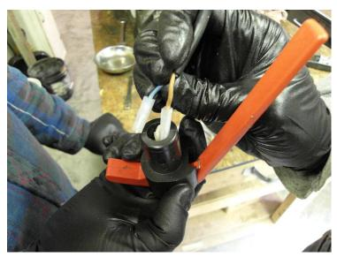
3) If the wires come out with the holder, pull them loose from the switch to disconnect.
