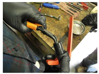
4) Remove switch from holder by holding white tab in center with pliers and un-screwing counter-clockwise.
