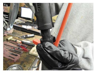
6) Push OPC lever holder with new switch and wires attached back into the end of the handlebar. Gently pull the slack out of the OPC wire you fed through the hole in the handlebar earlier. Don't pull too hard, or you'll unhook the terminals!
