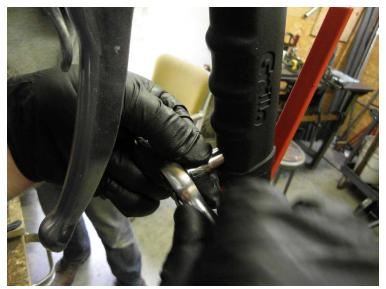
7) Reinstall screw (with 7mm socket), securing the OPC lever holder to the handlebar.
